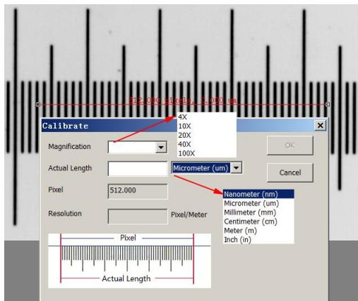
6. Try to align the two ends of the red line with the video ruler scale (Try to pull the
